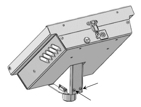
Pole impacts from snow removal equipment or errant vehicles can cause the, at the top of a 12-14 foot, the control unit to whip, damaging the neck rivets.
