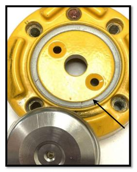
There is very little room between the outer circumference of the silver dome and the recessed deck of the body of the Bull Dog. When we removed the silver dome we did notice a very thin line of what looks like silicon around it. It is expected this is / was acting similar to a gasket. Closer inspection to the silicon we could see some irregularity to its uniformity - this could have been damage from
